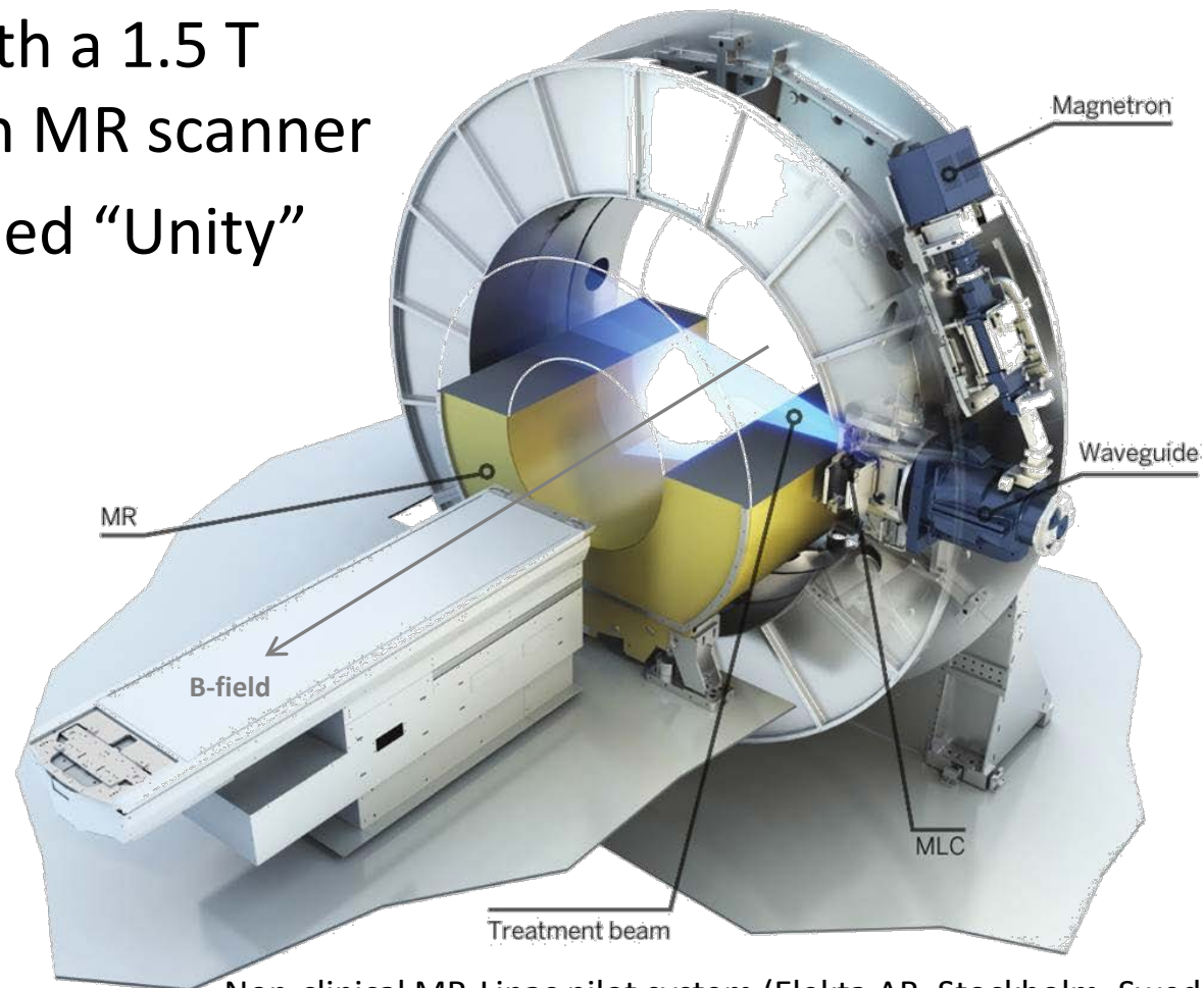
Non-clinical MR-Linac pilot system (Elekta AB, Stockholm, Sweden)
